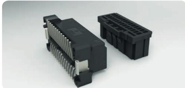
DYNAMIC SMT connectors are designed to meet the growing demand for a reliable, low cost, reflow solder capable part. Special designed retention legs increase the strength on the circuit board. The SMT type can withstand a maximum temperature of 245°C.
