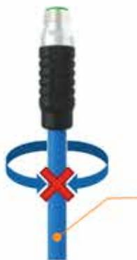
Crimping the cable jacket prevents cable rotation which is likely to occur in a cable gland. This can potentially lead to breakage of the conductors in the cable. Which are very difficult to find.
